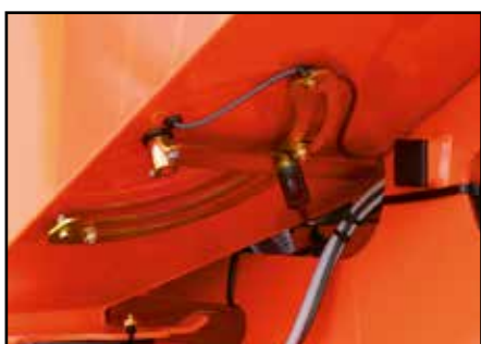
An electronic low level sensor, adjustable from outside the tank, monitors a range of seeds from small quantities of rape to bigger seeds and larger quantities.
