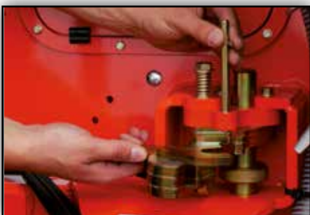
Adjustment of the central wheel by spacer
