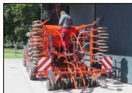
The loading steps and platform provide safe access for filling and inspection of the hopper.
