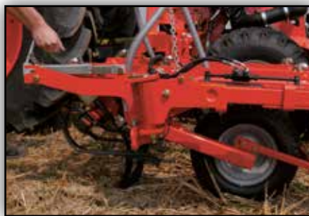
Adjustment of the lateral control wheels
