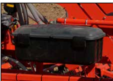
The rotors, when not in use, are always ready to hand stored well protected against dust in a toolbox. There is also a calibration bag and scale.
